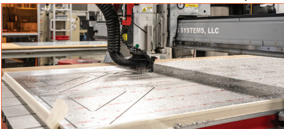
Pacer CNC Router: (x144" Y60" Z6.5") VAC table Tecno Router: (X120" Y60" Z3") VAC table
